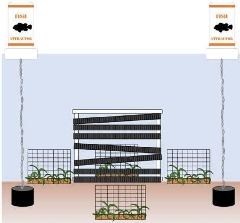
FIGURE 17.—NCSU vegetated fish attractor structure, including vegetation and artificial submersed cubes.
